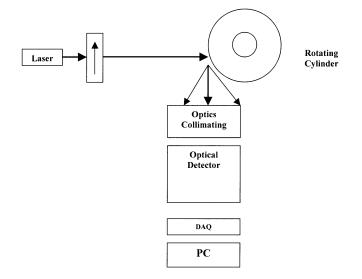
Fig. 2. Light intensity detection experimental setup.
