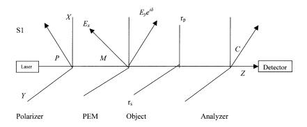
Fig. 1. Optical beam polarization pathway in the experiment setup.
