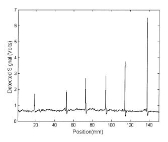
Fig. 11. Normalized first harmonic signal, 50.17 kHz, of the detected signal, for different wires of diameter of 0.1016, 0.1143, 0.160 02, 0.2032, 0.254, and 0.3048 mm using polarimetric detection technique.
